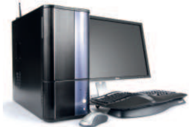
› The Ultimate Linux Box from LXF92 had a 1kW power supply, but that's a maximum – once the power saving was set up correctly, the machine draws only about a tenth of that.
