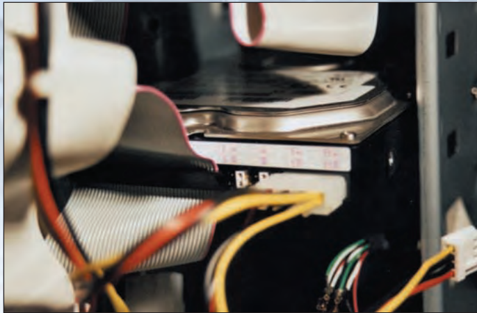
Figure 5: A close up of the hard disk and its jumper and cabling.
